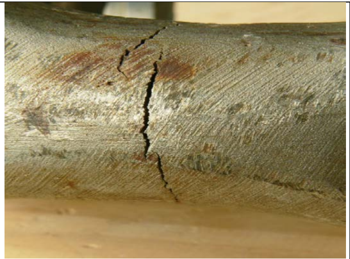
Image showing the cracks at the Bow end of the shackle
